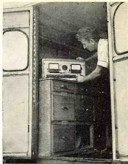
A "must" for two-way service is a monitor like the Motorola unit shown in use here. It measures modulation deviation and r.f. carrier-frequency departure directly in kilocycles.
